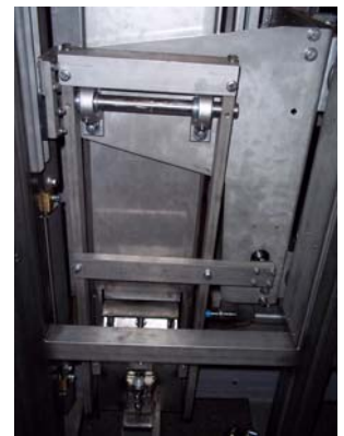
Lift Assembly w/ stainless steel bearings
