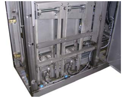
Lift Assembly w/ stainless steel bearings
